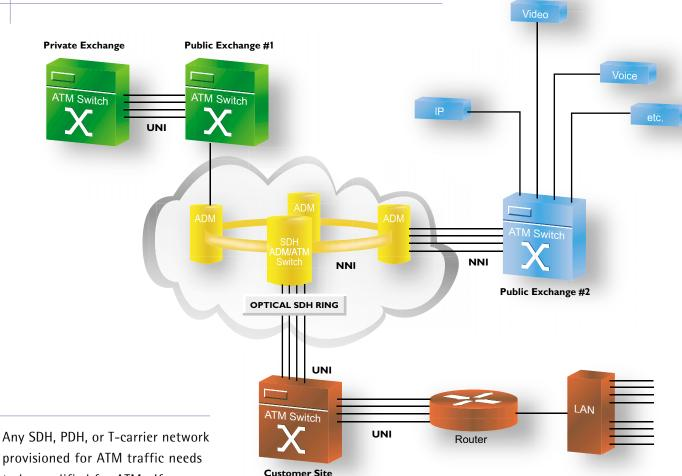
provisioned for ATM traffic needs to be qualified for ATM. If you lease your network to service providers using ATM, you need a tool to test, verify and troubleshoot the network and the traffic it is carrying. Conversely, if you are responsible for the ATM traffic, you must verify that the network is error free and functioning properly, especially when you do not own the network. When traffic is disrupted, you cannot waste valuable time and money pointing fingers.
