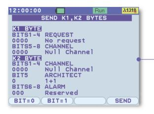
Advanced users can control/read SDH overhead bytes. The english decodes make overhead simple.
